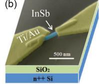
Fig. 1 (a) Representative SEM image (30° tilted angle view) of the as-grown nanowire sample, illustrating from top to bottom the AuIn<sub>2</sub> seed particles, the top InSb segments, and the thinner InAs stems, respectively. (b) SEM image (in false colors) of a typical InSb nanowire device contacted by Ti/Au and schematic view of the Si/SiO<sub>2</sub> substrate on which the device is fabricated. An InSb nanowire quantum dot is formed between the two Ti/Au contacts at low temperatures.
