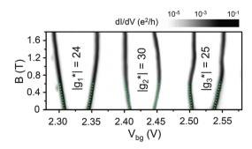
Fig. 4 Gray scale plot of magnetic field evolution of the differential conductance  $dI_{\rm ds}/dV_{\rm ds}$  measured in the linear response regime (i.e., at bias voltage  $V_{\rm ds}=0$  V) for the same quantum dot device as in Fig. 3. The g factors extracted from the measurements for quantum levels are indicated in the figure. The green dashed lines denote the data used to extract the g-factors.
