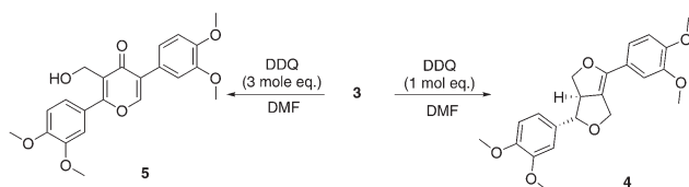
Scheme 2 Synthesis of pyran-4-one 5 from eudesmin ( 3 ).
