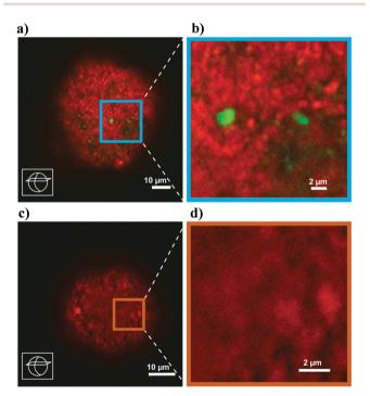
Fig. 27 Confocal fluorescence microscopy images showing the visualization of zeolite Y aggregate domains within an FCC catalyst particle with (a and b) and without (c and d) zeolite material. The images were obtained after reaction with thiophene (green) at 373 K and subsequent staining with Nile Blue (red) at 298 K. Images b and d are magnified views of the highlighted areas in a and c, respectively. (Reproduced with permission from ref. 175, Copyright Macmillan Publishers, 2011).
