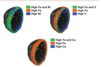
Fig. 26 Comparison of clustering masks for the metal poisons Fe, Ni, V and Ca for an individual E-cat FCC catalyst particle for the correlation pairs Fe/Ni, Fe/V and Fe/Ca as determined with X-ray micro-fluorescence tomography. (Redrawn from ref. 174).
