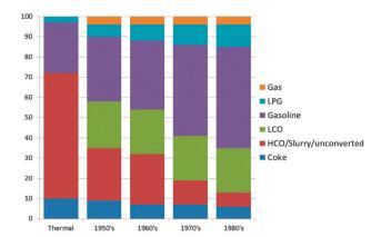
Fig. 2 The effect of improving reactor and catalyst technology on the product selectivity for the FCC process for four decades in the 1900's. Color-coding: gas: orange; LPG: light blue; gasoline: purple; LCO: green; HCO/slurry/unconverted: red; and coke: dark blue. Data are obtained from ref. 15 and 16.
