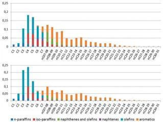
Fig. 15 A comparison of the total products from the same runs as depicted in Fig. 4. The graphs are combinations of the GC × GC plot for total liquid product, PIANO analysis of the naphtha fraction, and GC analysis of the gases. Top: Products from a normal cracking run. Bottom: Products with ZSM-5 containing additive added to the catalyst. Colorcoding: n-paraffins: dark blue; iso-paraffins: red; naphthenes and olefins: green; naphthenes: purple; olefins: blue; aromatics: orange.
