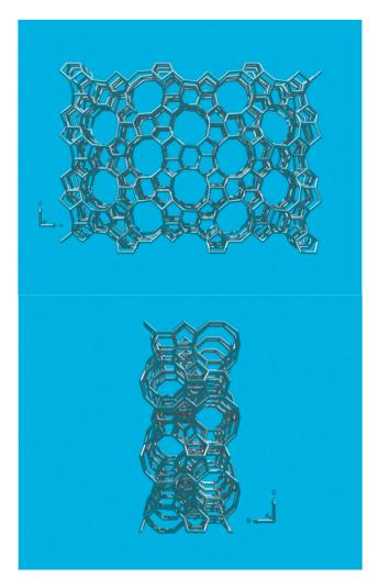
Fig. 14 (Top) Structure of zeolite ZSM-5, viewed along the 10-MR straight channels. (Bottom) View along the zig-zag channels.
