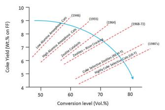
Fig. 11 Effect of subsequent developments in active components on conversion and coke level. Redrawn from ref. 65.
