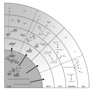
Consecutive cracking reactions of complex feedstock leading to the final FCC products. (Reproduced from ref. 32 with permission, Copyright Elsevier, 2005).
