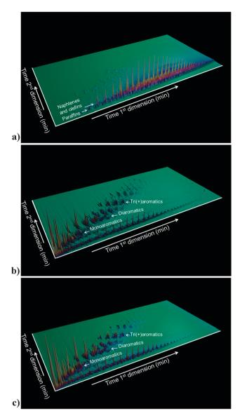
Fig. 5 (a) GC  $\times$  GC plot of a typical FCC feedstock (i.e., VGO). (b) GC  $\times$  GC plot of the products of cracking the VGO in (a), making use of an FCC catalyst with zeolite Y. (c) GC × GC plot of the products of cracking the VGO making use of an FCC catalyst with zeolite Y in the presence of zeolite ZSM-5 as additive.
