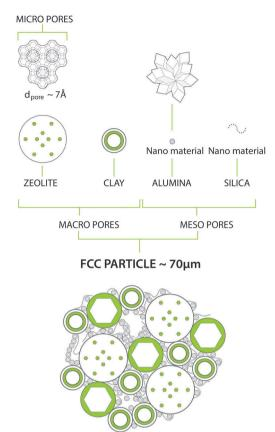
Fig. 7 Typical chemical and structural composition of a FCC particle. Artwork by RSK Communication.
