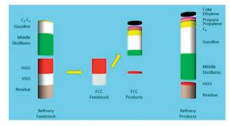
**Fig. 6** The effect of FCC conversion on total refinery product. Left: Atmospheric distillation frees up about 50% of the feedstock (middle distillates, gasoline and light gases). Heavy gas oil (HGO) and vacuum gas oil (VGO) are converted in the FCC unit. The products from FCC are combined with the initial products from crude distillation in the column on the right. More recent FCC processes will also convert part of the residue. Data from ref. 31.
