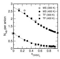
Fig. 12 Average number of hydrogen bonds accepted by the triflate- and methylsulfonate-ions at 300 K and 400 K, respectively
