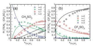
Fig. 15 Percentage of methylsulfonate- (a) and triflate-ions (b) hydrogenbonded to zero, one, two, and three TEA-cations, as a function of the mixture-composition at 400 K. Symbols: MD-simulation. Solid lines: model using equal statistical weights with  $w_{6,n} = 1$  for  $n \le 3$  and  $w_{6,n} = 0$
