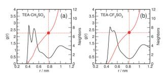
**Fig. 4** Anion–cation center of mass pair distribution functions g(r) obtained for (a) pure TEAMS and (b) pure TEATF at T=300 K. The position of the first minimum is used as a cut-off distance for the nearest neighbor computation (TEA–MS: 0.78 nm, TEA–TF: 0.81 nm).
