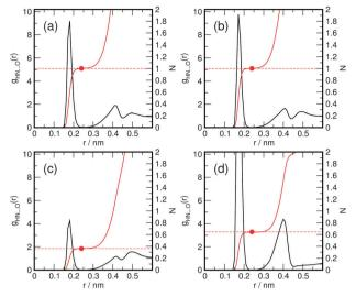
**Fig. 8** H-O intermolecular site-site radial pair distribution functions g(r) obtained for pure TEATF and TEAMS ionic liquids and their 50:50 mixture at 300 K. Also shown are the number of nearest neighbors as a function of distance N(r). (a) pure TEATF (b) pure TEAMS (c) H-O correlation between TEA and TF in the  $x_{\rm MS}=0.25$  mixture (d) H-O correlation between TEA and MS in the  $x_{\rm MS}=0.25$  mixture.
