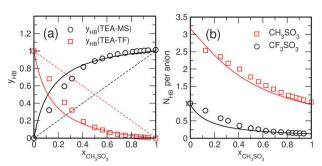
Fig. 16 (a) Percentage of TEA-cations connected via a hydrogen bond to either a triflate-ion or a methylsulfonate-ion as a function of the mixture-composition. (b) Average number of hydrogen bonds accepted by the triflate- and methylsulfonate-ions. Open symbols: MD-data obtained at 400 K. Solid lines: model using equal statistical weights with  $w_{6,n} = 1$  for  $n \le 3$  and  $w_{6,n} = 0$  for n > 3.
