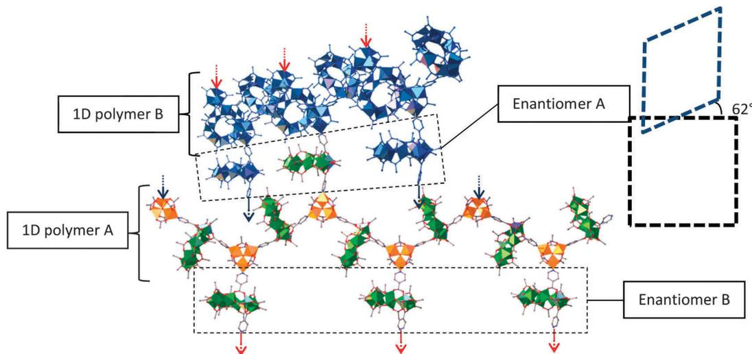
**Fig. 3** Showing the 1D chains and crosslinking within the framework. Colours as Fig. 2. Blue chain represents neighbouring polymer chain. The red and blue arrows represent where the crosslinks of each chain bind to the polymers in the neighbouring planes. The dashed boxes represent the angle of offset between the chains in the neighbouring planes.
