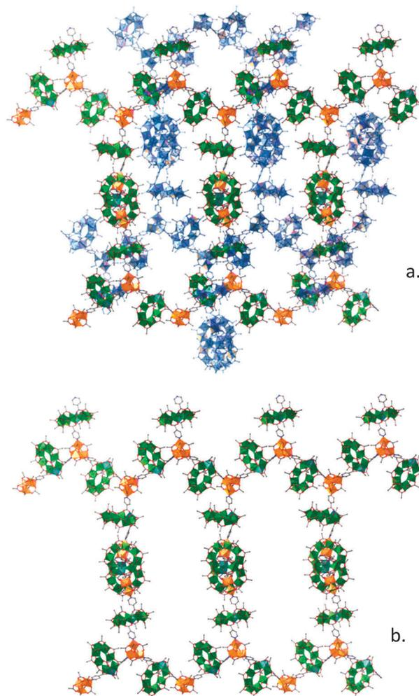
Fig. 2 (a) Orthographic view of **5** with one net coloured light blue to highlight interpenetrated nature. (b) Showing a single net. *t*-Butyl groups of pivalate groups and central ammonium cations removed for clarity. Green = chromium, turquoise = nickel, orange = iron/cobalt, grey = carbon, red = oxygen, blue = nitrogen, yellow = fluorine.
