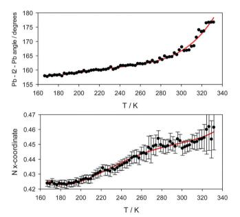
Fig. 5 Top – variation in the Pb–I2–Pb angle as a function of temperature in the tetragonal phase. Bottom - methylammonium nitrogen atom x-coordinate over the same temperature range.
