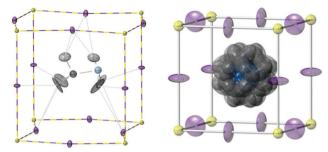
Fig. 2 Left: one orientation of the MA<sup>+</sup> cation in the tetragonal phase of MAPbl<sub>3</sub> at 180 K; the cation is four-fold orientationally disordered around the c-axis which is vertical in this diagram. Right: orientational disorder modelled in the cubic phase at 352 K. Atom key as in Fig. 1 and ADP ellipsoids at 50% probability.
