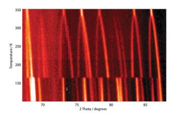
Fig. 3 Stacked plot, viewed vertically, of part of the NPD data (67-88°) collected from MAPbl<sub>3</sub> over the temperature range 100-352 K. Peaks are shown as white and pale orange on a black background. The phase changes at 165 and 327 K are clearly observed as is the overall unit cell expansion.
