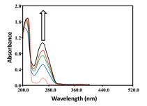
Fig. 4 Absorption spectra of L1 (1.6  $\times$  10<sup>-4</sup> M) in the absence (red dashed line) and presence (solid lines) of increasing DNA concentrations; 0.5  $\times$  10<sup>-4</sup> M (blue), 0.8  $\times$  10<sup>-4</sup> M (green), 1.1  $\times$  10<sup>-4</sup> M (red) and 1.4  $\times$  10<sup>-4</sup> M (black). Arrow indicates the hyperchromic shifts with increasing DNA concentrations (0.5–1.4  $\times$  10<sup>-4</sup>).
