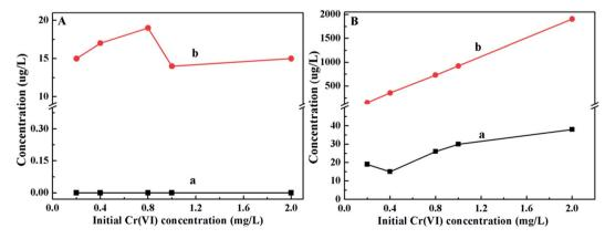
Fig. 6  $Cr(v_1)$  (a) and total Cr (b) concentrations in the solution (A) and PANI/CFs (B) after adsorption with initial  $Cr(v_1)$  concentrations ranging from 0.2 to 2.0 mg  $L^{-1}$ .
