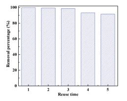
Fig. 8 Cr( $v_1$ ) removal efficiency of the regenerated PANI/CFs after 60 min adsorption. ([Cr( $v_1$ )]: 4.0 mg L $^{-1}$ , [PANI/CF]: 55.0 mg, pH: 1.0, treating time: 60 min).
