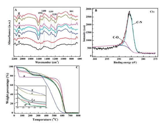
Fig. 2 (A) FT-IR spectra of the (a) as-received CFs, (b) CFs washed by HNO<sub>3</sub>, PANI/CFs with a PANI loading of (c) 5.0, (d) 10.0, (e) 15.0, (f) 20.0 wt%, and (g) pure PANI; (B) XPS C1s spectra of the synthesized PANI/CFs with a PANI loading of 10 wt%; and (C) TGA curves of (a) the as-received CFs, (b) CFs washed by HNO<sub>3</sub>, PANI/CFs with a PANI loading of (c) 5.0, (d) 10.0, (e) 15.0, (f) 20.0 wt%, and (g) pure PANI, respectively.
