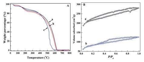
Fig. 7 (A) TGA curves of PANI/CF (a) before and after treating with (b) 8.0 and (c) 32.0 mg  $L^{-1}$  Cr(vi) solution; (B) the nitrogen adsorption–desorption isotherm of PANI/CFs with a 10.0 wt% loading after treated with (a) 4.0 and (b) 12.0 mg  $L^{-1}$ .
