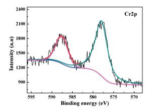
Fig. 5 XPS Cr2p spectra on PANI/CFs after the adsorption of Cr(vı) solution with an initial concentration of 48.0 mg  $\rm L^{-1}$  and pH of 1.0.
