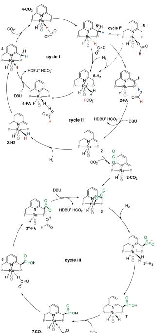
Scheme 2 Possible catalytic cycles for CO<sub>2</sub> hydrogenation to formates by Ru-PNP pincer complexes (\*Bu substituents of the ligand are omitted for clarity).
