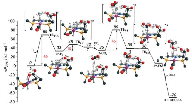
Fig. 7 DFT computed reaction energy diagram and optimized structures of the intermediate and transition states (CH<sub>3</sub> groups at the <sup>t</sup>Bu substituents of the PNP ligand are omitted for clarity) for the direct hydrogenation of CO2 over 3 (cycle III).
