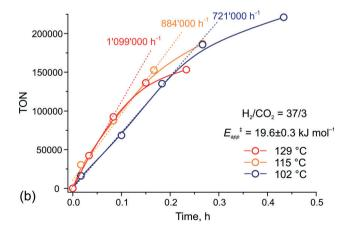
Fig. 9 Kinetic traces for CO<sub>2</sub> hydrogenation by 1 at different temperatures and  $H_2$ – $CO_2$  ratio of (a) 3/1 and (b) 37/3 ( $p_{total}$  = 40 bar).
