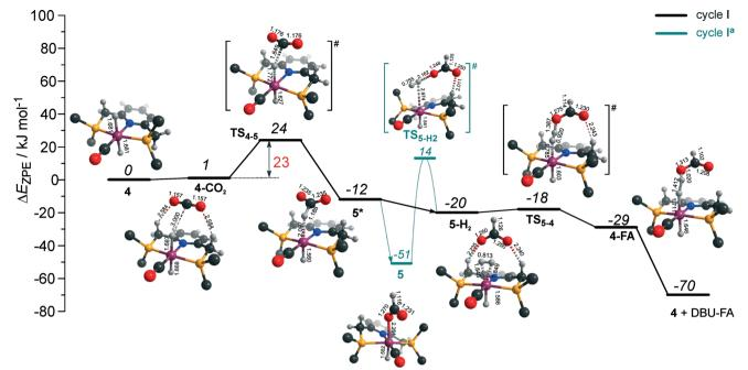
Fig. 3 DFT computed reaction energy diagram and optimized structures of the intermediate and transition states (CH<sub>3</sub> groups at the <sup>t</sup>Bu substituents of the PNP ligand are omitted for clarity) for the hydrogenation of CO<sub>2</sub> over 4.47
