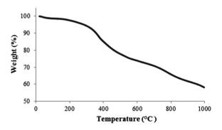
Fig. 4 TGA curve of MNPs 7.
