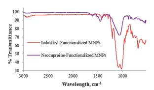
Fig. 2 FR-IR spectra of iodoalkyl-functionalized SiO<sub>2</sub>-coated MNPs **3** and neocuproine-functionalized SiO<sub>2</sub> coated MNPs **7**.
