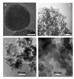
Fig. 3 TEM images of (a, b)  $\gamma$ -Fe<sub>2</sub>O<sub>3</sub> MNPs **1**, (c) iodoalkyl-functionalized SiO<sub>2</sub>-coated MNPs **3** and (d) neocuproine functionalized MNPs **7**.
