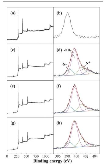
Fig. 2 XPS wide scan and N 1s core level spectra of pure PAN nanofibers (a and b), and PAN/PANI nanofibers prepared at different polymerization temperatures: 0 °C (c and d), 16 °C (e and f), 35 °C (g and h).
