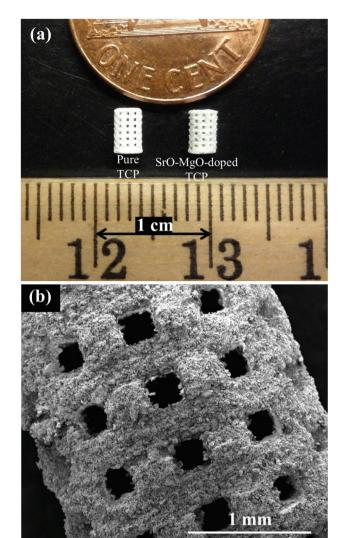
Fig. 2 (a) Photograph of the microwave sintered TCP and Sr-Mg doped TCP scaffolds, and (b) a high magnification SEM image of the pure TCP scaffold.
