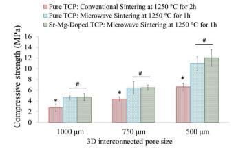
Fig. 5 Compressive strength comparison of 3DP microwave sintered Sr-Mg doped TCP scaffolds with the previously reported<sup>8</sup> microwave sintered and conventionally sintered pure TCP (\*p < 0.05, conventionally sintered pure TCP vs. microwave sintered pure and Sr-Mg doped TCP; #p > 0.05, microwave sintered pure TCP vs. Sr-Mg doped TCP; n = 10).
