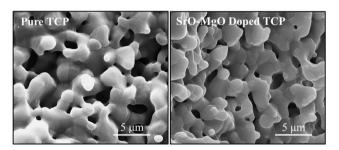
Fig. 4 Surface morphology of microwave sintered 3DP pure TCP and SrO and MgO doped TCP scaffolds.
