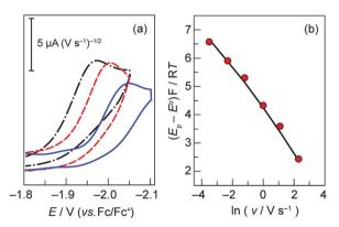
Fig. 2 (a) Overlay of representative CVs taken of a 0.2 mM solution of 1 in acetonitrile with 0.03 (—•), 0.3 (—•), and 3 (——) V s<sup>-1</sup> scan rates, using a glassy carbon electrode. (b) Plot of  $(E_p - E^\circ)$  F/R T vs. In of scan rate  $(E^\circ = -2.14 \text{ V}$ , taken from system 2). Experimental data (•), simulated curve (——) plotted for  $k_s = 0.24 \text{ cm s}^{-1}$  and  $k_{PT} = 8.5 \times 10^6 \text{ s}^{-1}$ .
