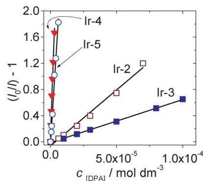
**Fig. 21** Stern–Volmer plots generated from phosphorescence intensity quenching of complex **Ir-2** ( $\lambda_{\text{ex}} = 386$  nm), **Ir-3** ( $\lambda_{\text{ex}} = 410$  nm), **Ir-4** ( $\lambda_{\text{ex}} = 475$  nm) and **Ir-5** ( $\lambda_{\text{ex}} = 425$  nm). Phosphorescence was measured as a function of DPA concentration in  $\text{CH}_3\text{CN}$ .  $1.0 \times 10^{-5} \text{ mol dm}^{-3}$ .  $20^\circ\text{C}$ . Reproduced with permission from ref. 45b.
