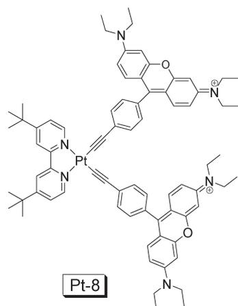
**Fig. 16** *N,N* Pt(II) acetylide complex containing rhodamine moiety. The complex shows strong absorption at 556 nm ( $\epsilon = 185\,800\text{ M}^{-1}\text{ cm}^{-1}$ ) and long-lived non-emissive  $^3\text{IL}$  excited state was observed ( $\tau_T = 83.0\text{ }\mu\text{s}$ ). The complex is from ref. 40.
