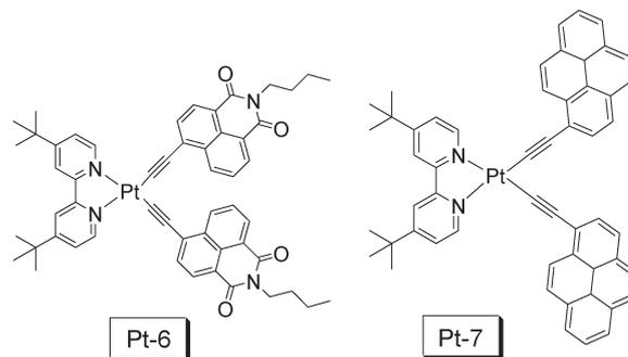
**Fig. 15**  $N^*N$  Pt(II) bisacetylide complexes that show prolonged  $T_1$  excited state lifetimes ( $\tau = 124.0 \mu\text{s}$  for **Pt-6** and  $\tau = 73.6 \mu\text{s}$  for **Pt-7**) used as triplet sensitizers for TTA upconversion. The compounds are from ref. 18 and 39, respectively.
