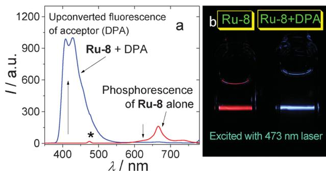
**Fig. 1** Illustration of the TTA upconversion. (a) Emission of the complex **Ru-8** (see Fig. 4 for molecular structure) and the upconversion with **Ru-8** as sensitizer and DPA as acceptor (see Fig. 2 for molecular structure). Excited by 473 nm laser. The asterisk indicates laser scattering. (b) Photographs of the upconversion samples of (a).
