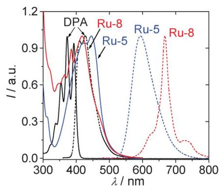
**Fig. 5** Normalized absorbance (solid lines) and emission spectra (dotted lines) of DPA, **Ru-5** and **Ru-8** in acetonitrile ( $1.0 \times 10^{-5}$  M). DPA,  $\lambda_{\text{ex}} = 380$  nm; **Ru-5**,  $\lambda_{\text{ex}} = 446$  nm; **Ru-8**,  $\lambda_{\text{ex}} = 418$  nm. 25 °C. Adapted from ref. 26 with permission.
