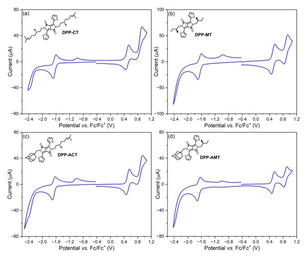
Fig. 3 Electrochemical investigation of chiral DPP dyes 1–4 in solution. Cyclic voltammograms of: (a) DPP-CT; (b) DPP-MT; (c) DPP-ACT; (d) DPP-AMT, recorded on a Pt disk (surface:  $0.07 \text{ cm}^2$ ) working electrode in CH<sub>2</sub>Cl<sub>2</sub>/n-Bu<sub>4</sub>NPF<sub>6</sub> 0.2 M solution. Sample concentration  $10^{-3}$  M; scanning rate 100 mV s<sup>-1</sup>.
