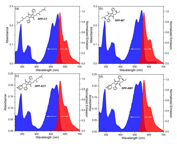
Fig. 2 Optical investigation of chiral DPP dyes 1-4 in CHCl<sub>3</sub> solution. Absorbance (blue) and photoluminescence (red) spectra of: (a) DPP-CT; (b) DPP-MT; (c) DPP-ACT; (d) DPP-AMT. For absorbance measurements: cell length 1 cm; sample concentration  $10^{-5}$  M. For photoluminescence measurements: sample concentration  $10^{-5}$  M, excitation wavelength 467 nm.
