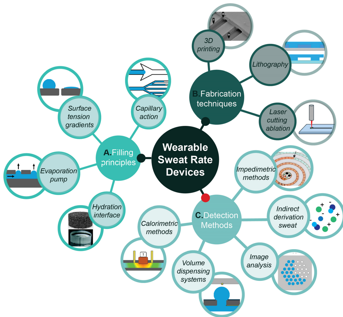
Fig. 1 Schematic overview of the A) filling principles, B) fabrication techniques and C) detection methods involved in the development of wearable microfluidic sweat rate devices. Reproduced with permission. 20–23 Hydration interface upper icon: Copyright 2024, Biomicrofluidics . Hydration interface lower icon: Copyright 2017, Lab Chip . 3D printing icon: Copyright 2017, Anal. Chem. Impedimetric methods: Copyright 2022, ACS Sens .
