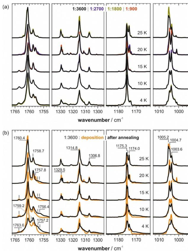
Fig. 3 (a) Experimental spectra of ITFE in an Ar matrix deposited at different temperatures and concentrations. The corresponding difference spectra are shown in Fig. S4 (ESI<sup>†</sup>). (b) Spectra of ITFE/Ar = 1:3600 after annealing at  $35\text{ K}$  with band markers for the signatures discussed in the text.
