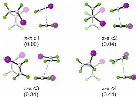
Fig. 4 The four lowest-energy dimeric structures of ITFE considered in the analysis of the experimental matrix-IR spectra. Relative energies (in kcal mol<sup>-1</sup>) obtained from single-point calculations at the DLPNO-CCSD(T) level of theory<sup>54,55</sup> on the revDSD-PBEP86-D3BJ optimized structures are given between parentheses.
