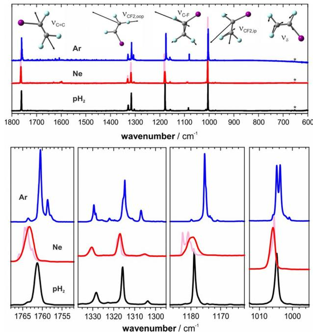
Fig. 1 Experimental IR spectra of ITFE recorded under different matrix-isolation conditions (*p*H<sub>2</sub>: 4 K, 1:1000; Ne: 4 K, 1:1800, two different depositions; Ar: 15 K, 1:1800). Top: Overview spectra and the displacement vectors corresponding to the five fundamental modes present in the experimentally accessible range. Bottom: Expanded views on the experimental spectra around the four strong fundamental transitions.
