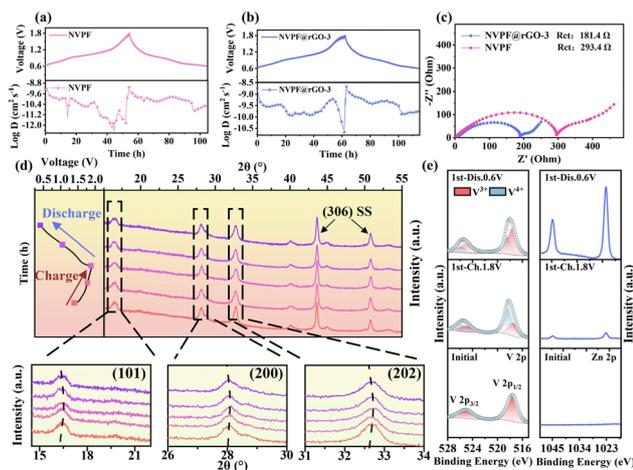
Fig. 4 GITT curves at 1C and the calculated diffusion coefficient of (a) NVPF and (b) NVPF@rGO-3. (c) Nyquist plots of NVPF and NVPF@rGO-3. (d) *Ex situ* XRD of NVPF@rGO-3. (e) *Ex situ* XPS of NVPF@rGO-3.
