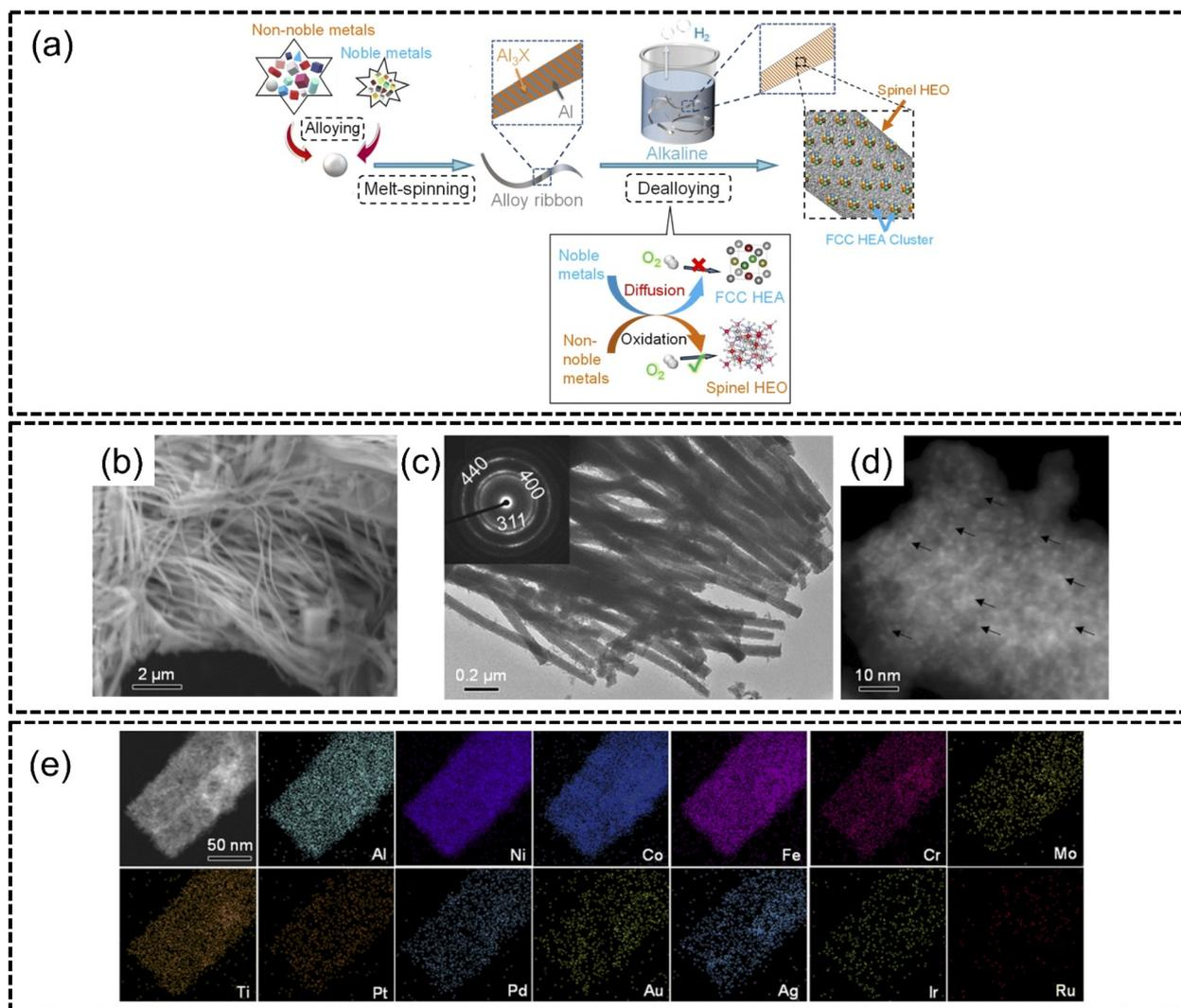
Fig. 9 Chemical dealloying synthesis from the work of Jin *et al.*, (a) schematic illustrations of the two-step alloying and dealloying of PtPdAuAgCuIrRu HEA on  $(\text{AlNiCoFeCrMoTi})_3\text{O}_4$  HEO, images of HEA cluster@HEO taken using (b) SEM, (c) TEM, (d) HAADF-STEM, and (e) STEM-EDX elemental mappings of the HEA cluster@HEO. The scale is 50 nm. Reproduced with permission.<sup>120</sup> Copyright Royal Society of Chemistry 2022.
