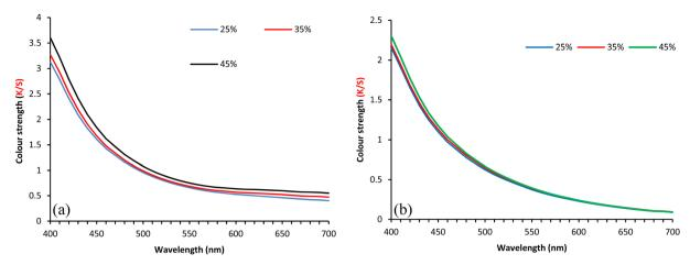
Fig. 4 Effect of Cu (a) and Ca (b), mordanting agent concentration (% ows) on the colour strength of the fabric dyed with 3% owf SL.
