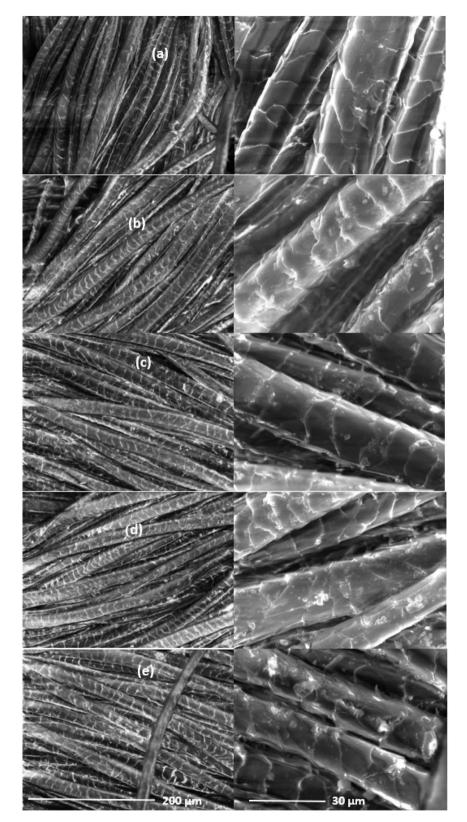
Fig. 8 SEM micrographs of surfaces of the control wool fabric (a), and also wool fabric samples treated with 5% owf SL using 25% ows Al (b), Ca (c), Cu (d), and Fe (e).
