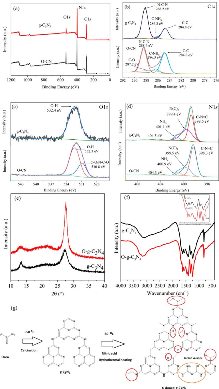
Fig. 1 (a) XPS survey spectra and short scan spectra of oxygen-doped  $g\text{-C}_3\text{N}_4$  with elements (b) C 1s, (c) O 1s, and (d) N 1s<sup>15</sup>; (e) XRD and (f) FTIR spectra of fabricated oxygen-doped  $g\text{-C}_3\text{N}_4$  (ref. 15); (g) ion exchange fabrication of oxygen-doped  $g\text{-C}_3\text{N}_4$ .<sup>17</sup>
