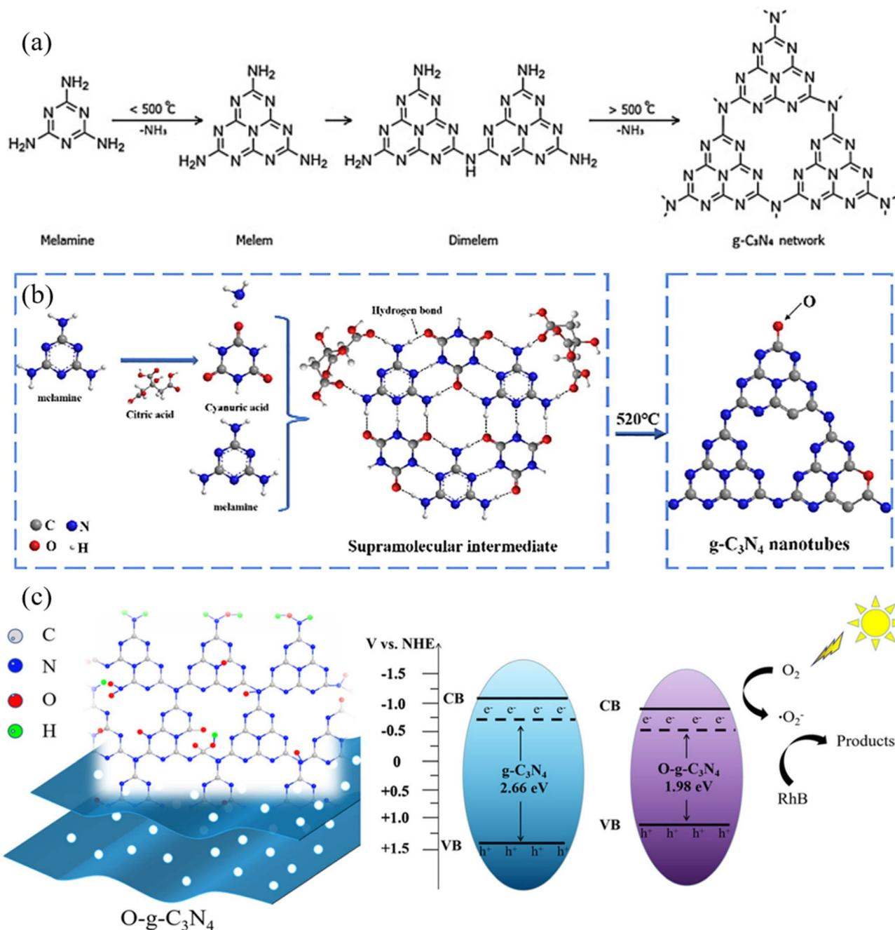
Fig. 2 Schematic illustration of structural changes during the synthesis of (a) g-C<sub>3</sub>N<sub>4</sub> (ref. 20) and (b) O@g-C<sub>3</sub>N<sub>4</sub> (ref. 23); (c) decrease in bandgap and increase in light absorption capacity due to oxygen doping onto g-C<sub>3</sub>N<sub>4</sub>.<sup>15</sup>
