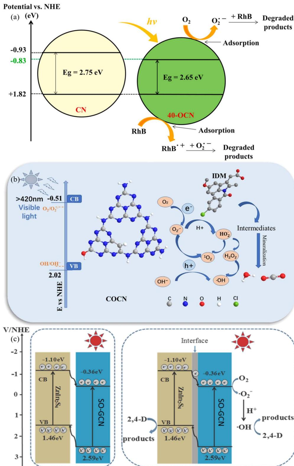
Fig. 3 (a) Degradation mechanism of pristine (a) O@g-C<sub>3</sub>N<sub>4</sub> (ref. 32), (b) O@g-C<sub>3</sub>N<sub>4</sub> developed on a 2D surface<sup>33</sup>, and (c) O@g-C<sub>3</sub>N<sub>4</sub>-based nanocomposite.<sup>34</sup>
