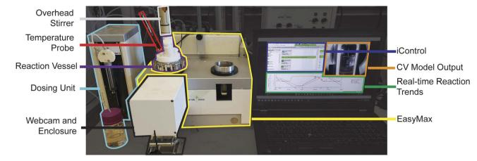
Fig. 2 Experimental workflow setup of *HeinSight 2.0*, illustrating the integration of EasyMax hardware components (dosing unit, overhead stirrer, temperature probe, and reaction vessel), webcam (within an enclosure), and software components ((CV model and iControl) with real-time trend visualization).
