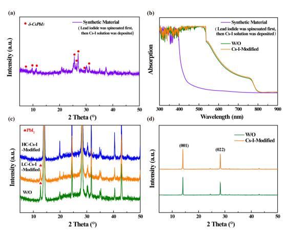
Fig. 2 (a) XRD patterns of the samples by reacting Pbl2 with equal molar Cs-I precursor solution; (b) UV-visible absorption spectra of the synthetic material, W/O and Cs-I-modified samples. XRD patterns for (c) the reference and films treated with low and high concentrations of the Cs-I precursor and (d) the W/O and Cs-I-modified perovskite films.
