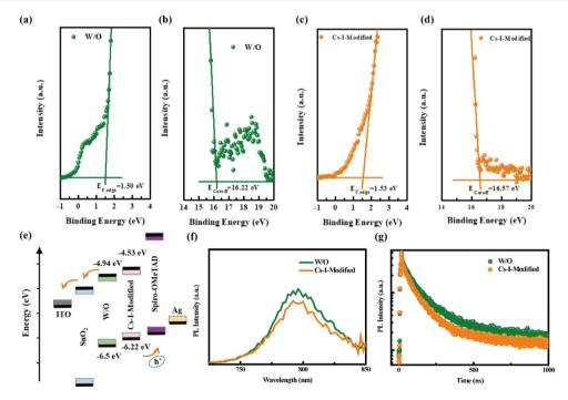
Fig. 4 The UPS spectra showing the  $E_{\text{cutoff}}$  and  $E_{\text{F,edge}}$  of (a), (b) the W/O film; (c) and (d) the Cs-I-modified film; (e) energy level diagram of device components. (f) PL spectra and (g) time-resolved PL spectra for the samples of Quartz/pristine PVSK/Spiro-OMeTAD and Quartz/Cs-I-modified PVSK/Spiro-OMeTAD.
