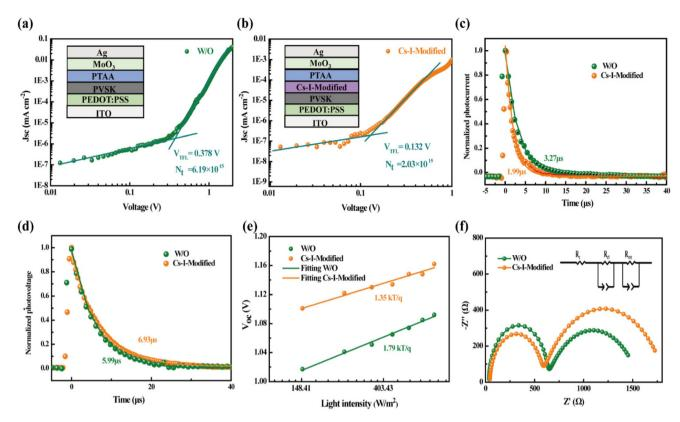
Fig. 5 Dark J-V curves of the hole-only devices with the structures of (a) ITO/PEDOT:PSS/Perovskite/PTAA/MoO<sub>3</sub>/Ag and (b) ITO/PEDOT:PSS/Cs-I-modified Perovskite/PTAA/MoO<sub>3</sub>/Ag. (c) TPC and (d) TPV decay curves, (e) V<sub>OC</sub> as a function of light intensities, and (f) Nyquist plots of the PSCs without and with Cs-I modification
