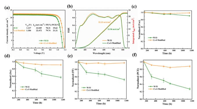
Fig. 6 (a) Comparison of J-V curves of the champion devices and their (b) EQE and corresponding integrated J<sub>int</sub> curves. The stability comparison of (c)  $V_{OC}$ , (d)  $J_{SC}$ , (e) FF, and (f) PCE of unencapsulated devices kept in the dark under a humidity of 15–25% RH at room temperature.
