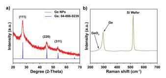
Fig. 2 (a) XRD pattern and (b) Raman spectra of Ge NPs.
