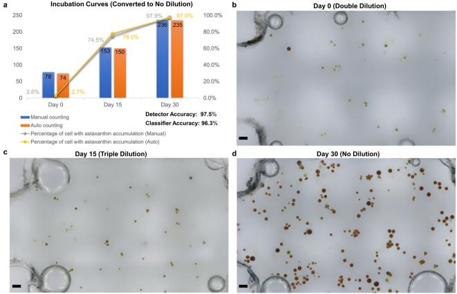
Fig. 5 Monitoring the accumulation of astaxanthin in Haematococcus Pluvialis. a) Culture experiment data and comparison graph of manual and AIMP obtained statistics. Example images of a single observation chamber at b) day 0 (samples are diluted twofold before adding to the chip), c) day 15 (samples are tripled diluted before adding to the chip), and d) day 30 (samples are not diluted). Scale bars are 200 µm.
