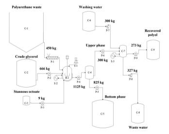
Fig. 19 Flow diagram of the split-phase glycolysis plant and mass balance per batch. Legend: C-1 = polyurethane silo; C-2, C-3, C-5, C-6, C-8 and C-9 = storage tanks; C-4 = decanter; C-7 = liquid-liquid extractor; R-1 = glycolysis reactor; E-1 = condenser; E-2 and E-3 = heat exchangers; P-1 = Archimedean screw; P-2, P-3, P-4, P-5, P-6 and P-9 = Gear pumps; P-7 and P-8 = centrifugal pumps. Reprinted from ref. 141 under Creative Commons Attribution 4.0 International License.
