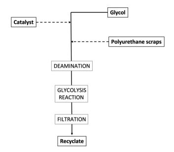
Fig. 10 Scheme of the glycolysis process for polyurethane wastes.
