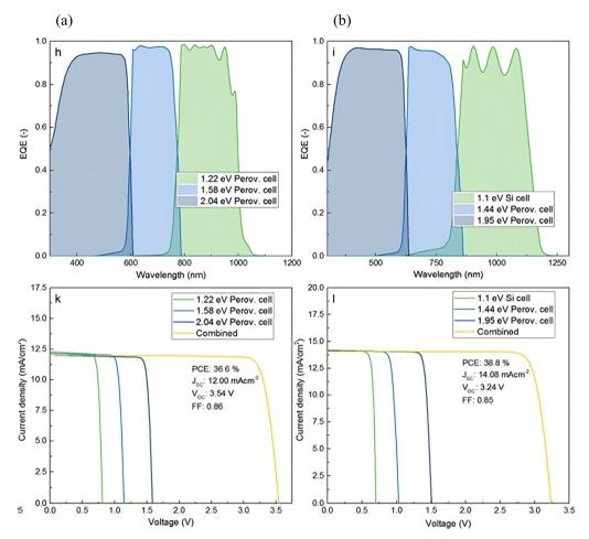
Fig. 4 Simulated external quantum efficiency (EQE) and current density-voltage (iV) curves for maximum practical PCE (a) 36.6% for an all-perovskite triple-junction solar cell with perovskite's bandgaps of 1.22 eV, 1.58 eV, and 2.04 eV for the subcells and (b) 38.8% for a perovskite/perovskite/silicon triple-junction solar cell with bandgaps of 1.44 eV and 1.95 eV for perovskite subcells. Reproduced with permission from ref. 27, Copyright © 2017, American Chemical Society
