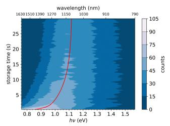
Fig. 6 Action spectra of laser-induced naphthalene-dimer dissociation,  $(C_{10}H_8)_2^+ \rightarrow C_{10}H_8^+ + C_{10}H_8$ . The intensity, as a function of the storage time before the firing of the laser and the laser photon energy, is shown through the color scale shown to the right. The red line is an exponential fit of the CR band position determined at maximum intensity, showing the shift of the CR band position with storage time.
