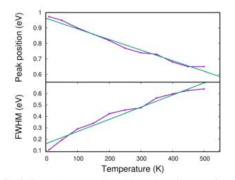
Fig. 13 Theoretical energy position of the maximum (upper panel) and width (lower panel) of the CR band as functions of temperature. The green lines are linear fits to the calculated data (see the text).
