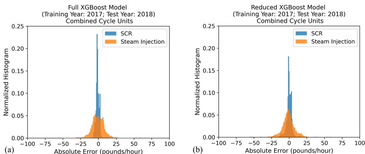
Fig. 6 The distribution of absolute errors, *i.e.*, the difference between the predicted NO<sub>x</sub> emission rates and the CAMD-derived NO<sub>x</sub> emission rates, for the combined cycle units with different NO<sub>x</sub> control technologies (with SCR, steam injection) output from the (a) full XGBoost model; (b) reduced XGBoost model trained on 2017 data and tested on 2018 data.
