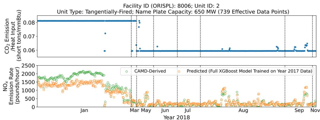
Fig. 7 The ratios between CO<sub>2</sub> emissions and heat input (upper), and CAMD-derived versus predicted NO<sub>x</sub> emission rates (bottom,  $R^2 = 0.86$ ) from Unit 2 of the Roseton Generating LLC facility in Newburgh, NY (Facility ID: 8006) in 2018, with abnormal high NO<sub>x</sub> emission rates in January corresponded with the under-prediction zone shown in the left scatter plot in Fig. 5a.
