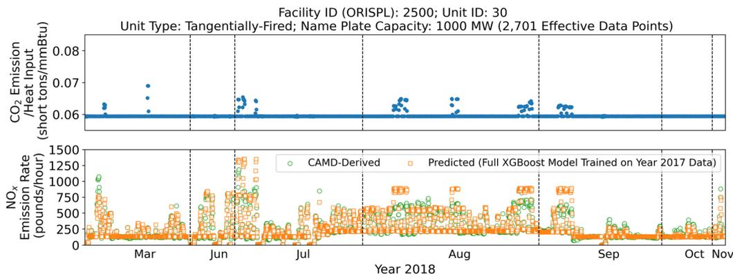
Fig. 8 The ratios between CO<sub>2</sub> emissions and heat input (upper), and CAMD-derived versus predicted NO<sub>x</sub> emission rates (bottom,  $R^2 = 0.88$ ) from Unit 30 of the Ravenswood Generating Station facility in Long Island City, NY (Facility ID: 2500) in 2018, with NO<sub>x</sub> emission rates of about 160 data points over-predicted in June, July, August and September corresponded with the over-prediction zone shown in the left scatter plot in Fig. 5a.
