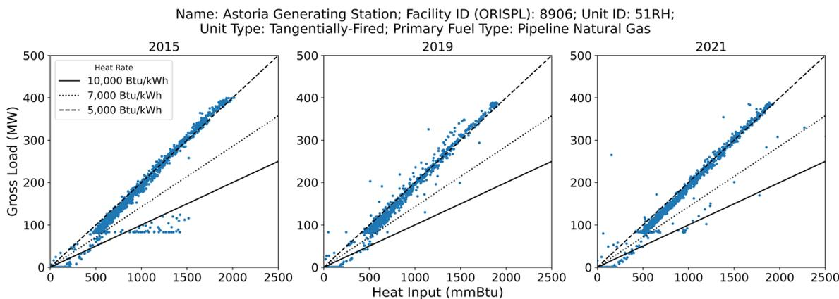
Fig. 2 The scatter plot of hourly recorded heat input *versus* gross load in 2015, 2019, and 2021, respectively, for the Unit 51RH at the Astoria Generating Station (Facility ID: 8906). Unit 51RH and Unit 52SH are two furnaces for the same boiler but the heat rates are reported by dividing the gross load for the full boiler by the heat input for each individual furnace, resulting in unrealistic values of around  $5000 \text{ Btu kW}^{-1} \text{ h}^{-1}$ .
