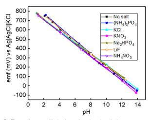
Fig. 7 The emf versus pH plot for various ions in solutions.
