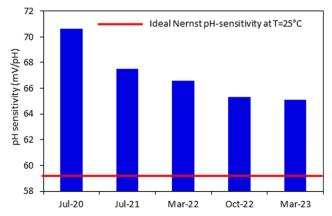
Fig. 9 pH sensitivity of fabricated electrodes over 32 months.
