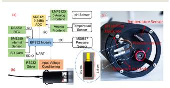
Fig. 1 (a) Block diagram (b) front-view and (c) bottom view of the underwater probe.
