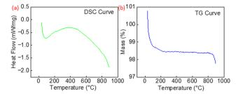
Fig. 4 (a) Heat flow (DSC curve) and (b) mass change (TG curve) for Co<sub>2</sub>O<sub>3</sub>-RuO<sub>2</sub> powder in the temperature range 20-900 °C.
