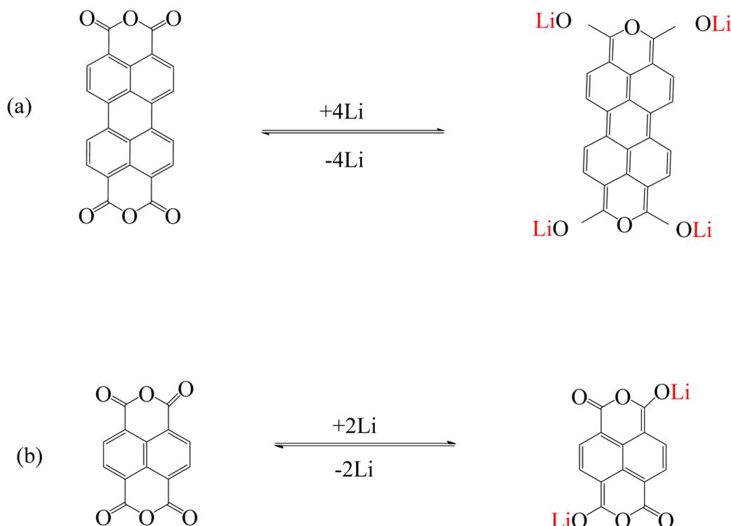
Fig. 6 Mechanism of lithium ion adsorption by (a) PTCDA (Reproduced with permission from ref. 87. Copyright 2023, Elsevier) and (b) NTCDA (Reproduced with permission from ref. 89. Copyright 2023, Royal Society of Chemistry).
