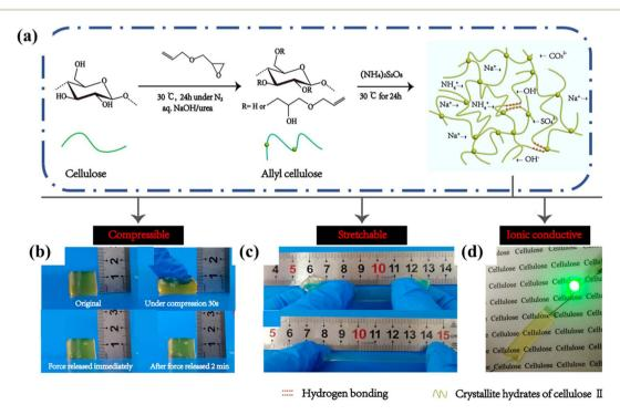
Fig. 12 (a) Schematic illustration of synthesis of cellulose hydrogels. Desirable properties include (b) compressibility, (c) stretchability, (d) ionic conductivity and transparency. Reprinted with permission from Tong et al.<sup>69</sup> Copyright 2019 American Chemical Society.
