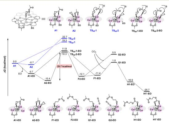
Scheme 6 Energy diagram for alternating copolymerization by neutral CaCo<sub>3</sub> complexes.
