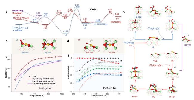
Fig. 3 (a) Free energy profiles (in eV) of  $CO_2HR$  on the  $Au_1/CeO_2$  SAC following pathways enabled by the LES (L-pathway) and HEMS (H-pathway). (b) Structures of all states. Configurations of  $CO_2$  activation on (c) the LES and (d) the HEMS. Calculated (e) turnover frequency (TOF) and (f) coverages of states as functions of temperature.
