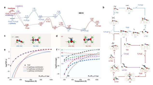
Fig. 4 (a) Free energy profiles (in eV) of SHA on the Pt<sub>1</sub>/CeO<sub>2</sub> SAC following pathways enabled by the LES (L-pathway) and the HEMS (Hpathway). (b) Structures of all states. Configurations of C<sub>2</sub>H<sub>2</sub> activation on (c) the LES and (d) the HEMS. Calculated (e) turnover frequency (TOF) and (f) coverages of states as functions of temperature
