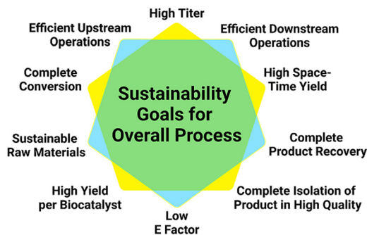
Fig. 7 Interconnected sustainability goals of various process parts (blue: up- and downstream processing parts; yellow: reaction engineering part) contributing to the sustainability of the overall process for metabolite synthesis.
