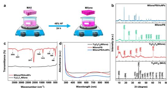
**Fig. 1** (a) Schematic diagram of the synthesis of  $Ti_3C_2T_x$  MXene from  $Ti_3AlC_2$  MAX phase by acid etching method. (b) XRD pattern of  $Ti_3AlC_2$  MAX phase,  $Ti_3C_2T_x$  MXene, MXene/PB, and MXene/PB/AuNPs nanocomposite. (c) FT-IR spectra of MXene and MXene/PB/AuNPs, and (d) UV-vis spectrum of MXene, MXene/PB, and MXene/PB/AuNPs.
