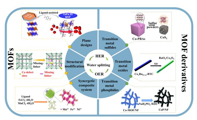
Scheme 1 Illustration of the main design strategies and types of MOFs and MOF derivatives in water splitting. Reproduced with permission. 60,66,75,83,88,91. Copyright 2019, RSC. Copyright 2019, Springer Nature. Copyright 2020, Wiley-VCH. Copyright 2017, RSC. Copyright 2017, RSC. Copyright 2020, RSC.
