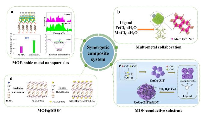
Fig. 3 Illustration of the synergetic composite system of MOF-based materials in electrocatalytic water splitting, (a) MOF-noble metal nanoparticles, (b) multi-metal collaboration, (c) MOF-conductive substrate and (d) MOF@MOF. Reproduced with permission: 70,71,75,76 Copyright 2023, Wiley-VCH. Copyright 2020, Wiley-VCH. Copyright 2020 Elsevier. Copyright 2018, Wiley-VCH.
