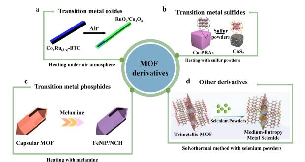
Fig. 4 Illustration of MOF derivatives including (a) transition metal oxides, (b) transition metal sulfides, (c) transition metal phosphides and (d) other derivatives in electrocatalytic water splitting. Reproduced with permission. 83,88,94,100 Copyright 2017, RSC. Copyright 2019 Springer Nature. Copyright 2020, RSC. Copyright 2019, American Chemical Society.
