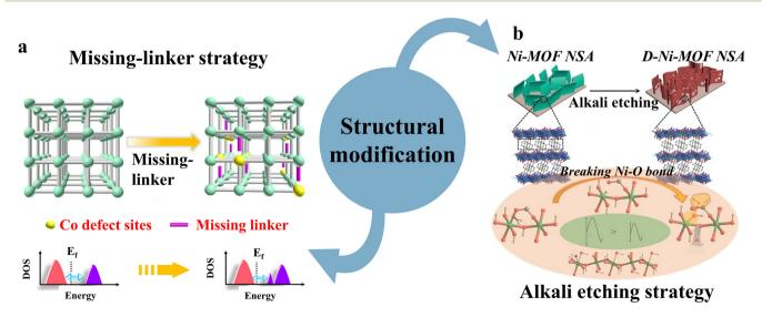
Fig. 2 Illustration of the structural modification strategies of MOF-based materials in electrocatalytic water splitting, (a) missing-linker strategy and (b) alkali etching strategy. Reproduced with permission. 66,67 Copyright 2020, Wiley-VCH. Copyright 2019 Springer Nature.
