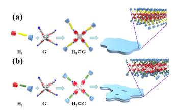
Fig. 10 Formation of host-quest complexes (a)  $H_1 \subset G$  and (b)  $H_2 \subset G$ , and self-assembly in CHCl<sub>3</sub>/DMSO solution, respectively.
