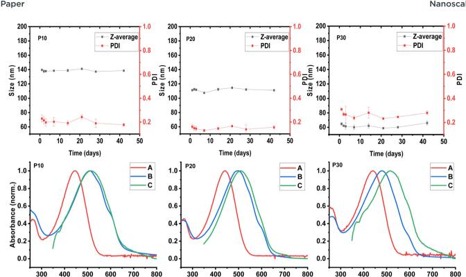
Fig. 2 (Top) Analysis of particle stability over time via DLS measurements from P10 (left), P20 (centre), and P30 (right) dispersions in water. (Bottom) UV-vis spectra of (A) polymer solutions in chloroform, (B) polymer dispersions in water and (C) thin films spin-cast from chloroform solutions, for P10 (left), P20 (centre), and P30 (right).
