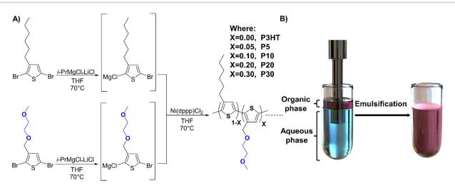
Fig. 1 (A) Schematic representation of the random copolymer synthesis. (B) Representation of the ultrasonication process to generate the corresponding surfactant-free polymer dispersion.
