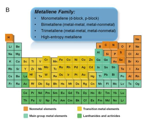
Fig. 1 (A) Schematic illustration showing three-generational development of 2D atomically thin materials including metal-free (X-ene, X = B, C, N, P, etc.), transition metal compounds (metal-X-ene, X = C, N, O, S, etc.), and metallic materials (metal-ene). (B) Overview of the elements involved in metallenes in the periodic table achieved by either experiments or theoretical calculations. (A) Reproduced from ref. 8 with permeation from CellPress. Copyright 2019
