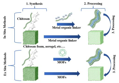
Fig. 6 Fabrication of CS/MOFs using different methods.
