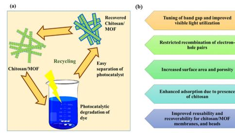
Fig. 11 (a) Pictorial representation of recycling CS/MOFs as a photocatalyst for the reclamation of dye wastewater under visible light. (b) The advantages of CS/MOFs as an efficient photocatalyst are also highlighted.
