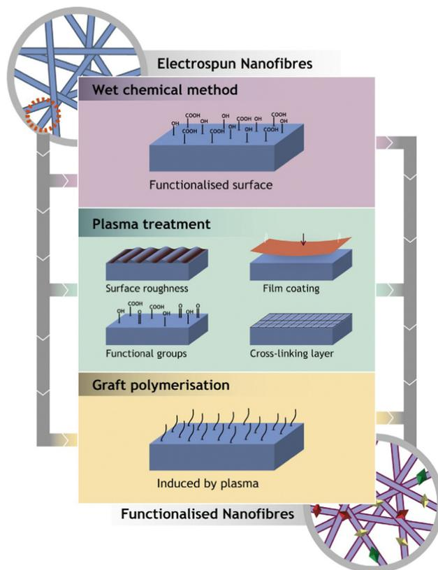
Fig. 4 Representation of the main surface modification techniques used to improve the surface nanofiber properties (reproduced with permission from ref. 83 ©2018 *Colloids and Surfaces B: Biointerfaces*, published by Elsevier Ltd).
