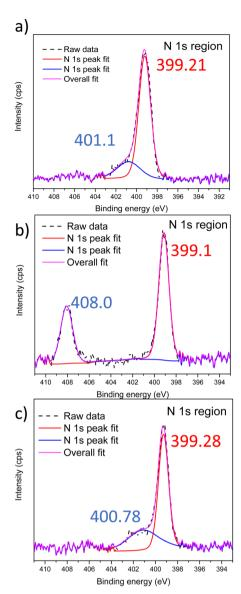
Fig. 2 XPS spectra in the N 1s region of (a) xLPSbP2VP/zwitterion, (b) xLPSbP2VP/alkoxy and (c) xLPSbP2VP/alkyl BCEs.
