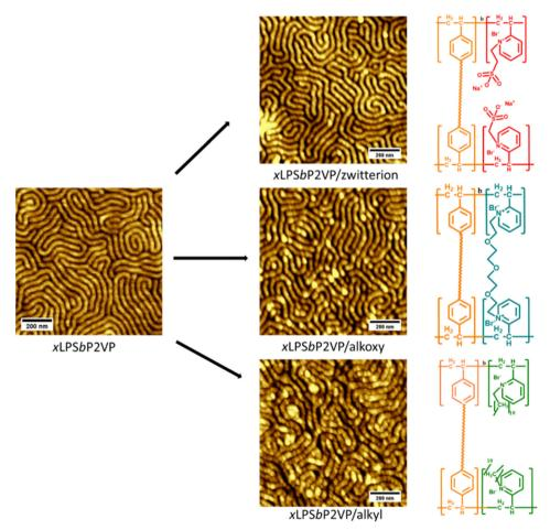
Fig. 1 AFM micrographs of xLPSbP2VP (left), xLPSbP2VP/zwitterion (top), xLPSbP2VP/alkoxy (middle), and xLPSbP2VP/alkyl (bottom) BCEs. The chemical structures of the BCEs are represented on the right side of their corresponding AFM image.
