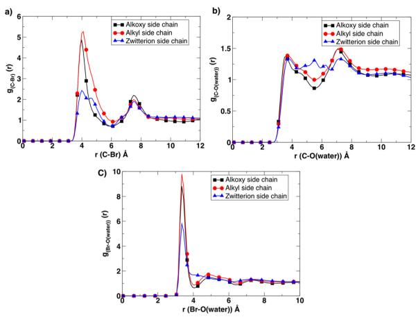
Fig. 4 The radial distribution function q(r) between (a) the C atom (the first methylene group of the side chain attached to the pyridinium N atom) and the bromide atom. (b) The C atom (the first methylene group of the side chain attached to the pyridinium N atom) and water O atom. (c) The radial distribution function g(r) calculated between the bromide atom and water O atom.
