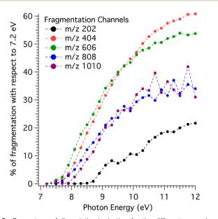
Fig. 5 Percentage of dissociative ionisation for the different mass channels obtained via the method outlined in Fig. 4, i.e., by comparison with the KERDs measured at 7.2 eV (7.5 eV for the m/z 202 channel).
