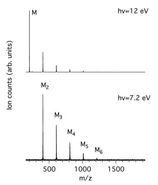
Fig. 1 Time-of-Flight mass spectra measured for photon energies of 7.2 eV (bottom) and 12 eV (top).
