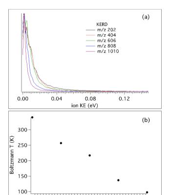
Fig. 3 (a) Ion KERDs up to the pentamer measured at a photon energy of 7.2 eV, except for the monomer which was acquired at 7.5 eV. (b) Translational temperatures extracted from (a) assuming a Boltzmann energy distribution
