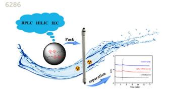
A C4-modified bipyridinium multi-mode stationary phase for reversed phase, hydrophilic interaction and ion exchange chromatography
