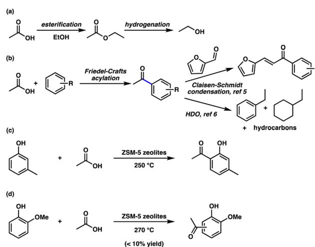
**Scheme 1** (a) Removal of acetic acid from fast pyrolysis-derived bio-oils by esterification and subsequent hydrogenation. (b) A strategy for removing acetic acid from fast pyrolysis-derived bio-oils by Friedel–Crafts acylation reactions. (c) Friedel–Crafts acylation reaction between *m*-cresol and acetic acid at 250 °C. (d) Friedel–Crafts acylation reaction between guaiacol and acetic acid at 270 °C.
