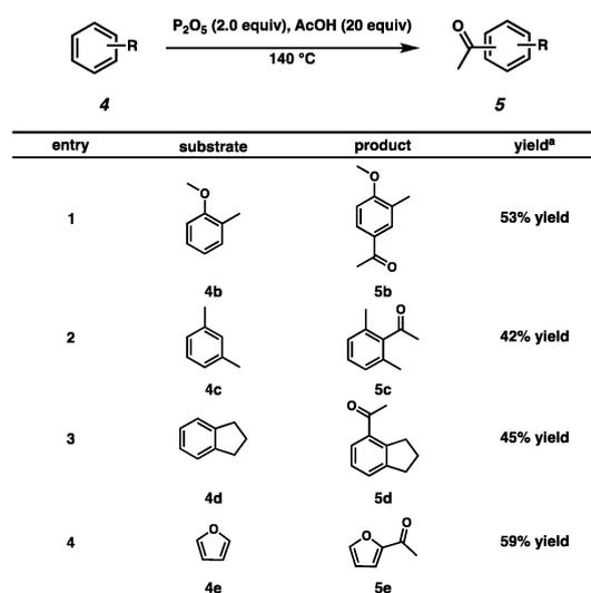
**Scheme 3** Friedel–Crafts acylation on non-phenolic components of fast pyrolysis-derived bio-oils (<sup>a</sup>Yield of the isolated product).
