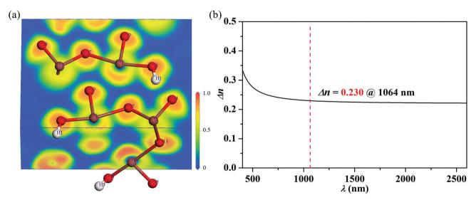
Fig. 5 (a) Electron localization function diagram and (b) calculated birefringence for  $Mg(H_2O)_6[(IO_2(OH))_2(IO_3)]_2$ .
