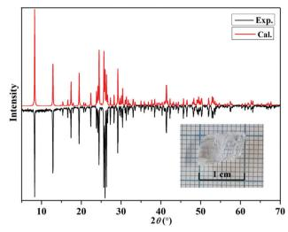
Fig. 1 Experimental and calculated powder XRD patterns of  $Mg(H_2O)_6[(IO_2(OH))_2(IO_3)]_2$ . Inset: The picture of an as-grown large crystal.
