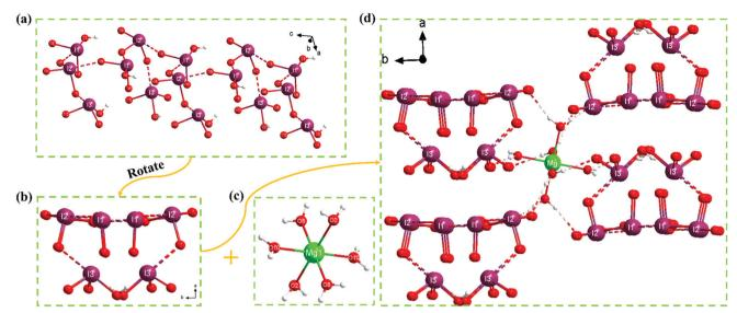
Fig. 2  $[(IO_2(OH))_2(IO_3)]^-$  infinite tubules viewed along the (a) b-axis and (b) c-axis, and the (c)  $[Mg(H_2O)_6]^{2^+}$  octahedron in  $Mg(H_2O)_6[(IO_2(OH))_2(IO_3)]_2$ . (d) Hydrogen bonding interactions between the  $[Mg(H_2O)_6]^{2^+}$  octahedron and  $[(IO_2(OH))_2(IO_3)]^-$  infinite tubules.
