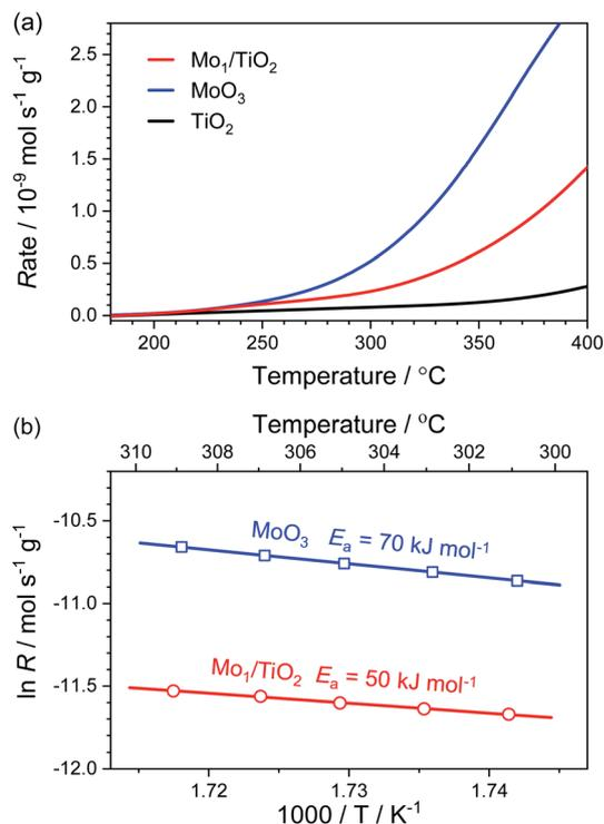
Fig. 4 (a) Reaction rates of the NH<sub>3</sub> oxidation as a function of temperature over Mo<sub>1</sub>/TiO<sub>2</sub>, MoO<sub>3</sub> and TiO<sub>2</sub>. (b) Arrhenius plots for reaction rates with E<sub>a</sub> over Mo<sub>1</sub>/TiO<sub>2</sub> and MoO<sub>3</sub>.
