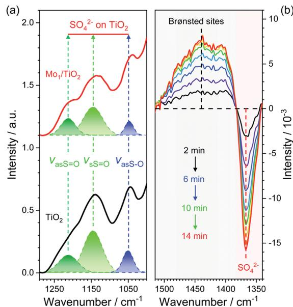
Fig. 5 (a) FT-IR spectra of ABS-deposited TiO<sub>2</sub> and Mo<sub>1</sub>/TiO<sub>2</sub>. (b) *In situ* DRIFT spectra of the transient reaction on the 0.5% ABS-deposited Mo<sub>1</sub>/TiO<sub>2</sub> catalyst at 260 °C. The initial spectrum was deduced as the background.
