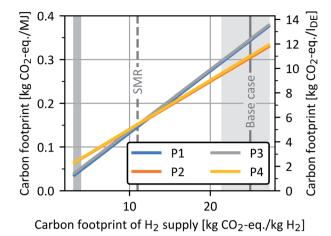
Fig. 15 Carbon footprint of all four OME<sub>3-5</sub> process routes as a function of the carbon footprint of H<sub>2</sub> supply. The left y-axis shows the carbon footprint in kg CO<sub>2</sub>-eq. per MJ, while the right y-axis additionally indicates the results in kg  ${\rm CO_2\text{-}eq.}$  per  ${\rm l_{DE}}$ . The shaded areas indicate the carbon footprint ranges of H<sub>2</sub> supply for the years 2018 (light grey) and 2050 (dark grey).68 SMR: steam methane reforming.
