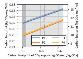
Fig. 14 Carbon footprint of all four OME<sub>3-5</sub> process routes as a function of the carbon footprint of CO<sub>2</sub> supply. The left y-axis shows the carbon footprint in kg  $CO_2$ -eq. per MJ, while the right y-axis additionally indicates results in kg CO<sub>2</sub>-eq. per l<sub>DE</sub>. The shaded areas indicate the carbon footprint ranges of CO2 supply from DAC (light grey) and MEA cement (dark grey) for the years 2018 and 2050.68
