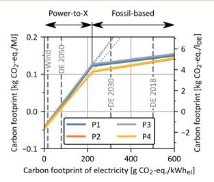
Fig. 13 Carbon footprint of all four  $OME_{3-5}$  process routes as a function of the carbon footprint of electricity supply for the base case. The left y-axis shows the carbon footprint in kg CO<sub>2</sub>-eq. per MJ, while the right y-axis additionally indicates results in kg  $CO_2$ -eq. per  $I_{DE}$ . Wind: wind power, DE 2018/2030/2050: German power grid mix 2018/2030/2050.68
