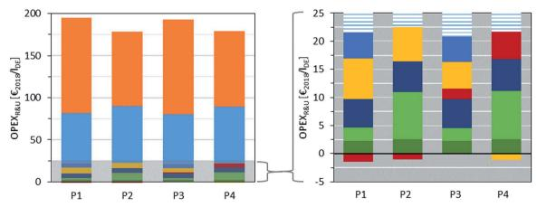
Fig. 8 Breakdown of raw material and utility R&U costs of routes P1-P4:  $\blacksquare$  H<sub>2</sub>,  $\blacksquare$  CO<sub>2</sub>,  $\blacksquare$  silver (FA, aqueous),  $\blacksquare$  20 bar steam,  $\blacksquare$  4 bar steam, ■ compressed air, ■ electricity, and ■ remaining costs.
