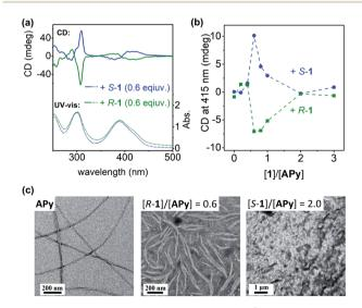
Fig. 4 (a) UV-vis and CD spectra of APy (6  $\times$  10  $^{-5}$  M) with 0.6 equiv. of S-1 and R-1. (b) Plots of CD at 415 nm for APy (6  $\times$  10<sup>-5</sup> M) upon addition of S-1 and R-1. All spectra were recorded in water at 25 °C. (c) TEM images of Apy (left), and mixtures of APy with chiral 1 ([R-1]/[APy] = 0.6 (middle); [S-1]/[APy] = 2.0 (right).
