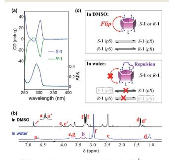
Fig. 2 (a) CD and UV-vis spectra of S-1 and R-1 (2  $\times$  10 $^{-5}$  M) in water. (b)  $^1$ H NMR spectra of S-1 (400 MHz) in D $_2$ O and DMSO- $d_6$ . All spectra were recorded at 25  $^{\circ}$ C. (c) Illustration of the unit flip of S-1 and R-1 in DMSO and inhibition of the unit flip in water.
